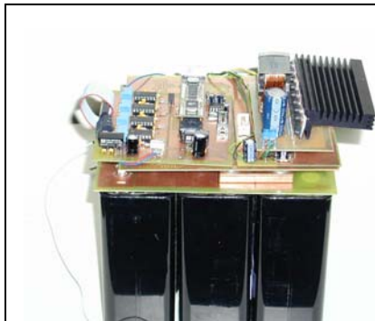
Figure 14: 14V UC storage with 400W DC/DC Converter
