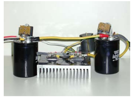
Figure 8: Buck / Boost converter
